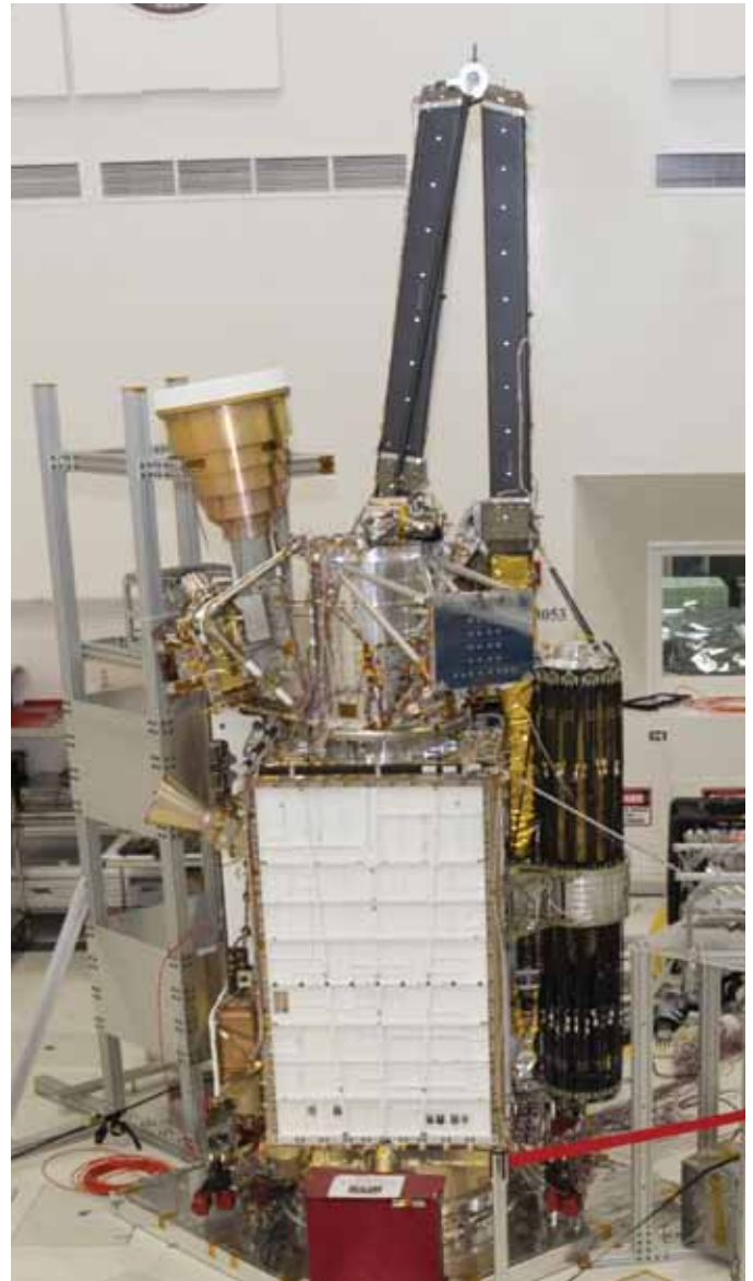
TOP RIGHT: The SMAP spacecraft and instrument, having just been put together into what is called the "Observatory" in January 2014. The spinning portion of SMAP's instrument system is seen mounted on top of the rectangular, box-like structure of the spacecraft. Prominently featured in the upper portion of the instrument and on its right-hand side are the deployable reflector antenna, which looks like a bundle of black-colored tubular elements, and the deployable boom above (also black in color), which will eventually support the antenna while spinning in space. Image Credit: NASA/JPL
