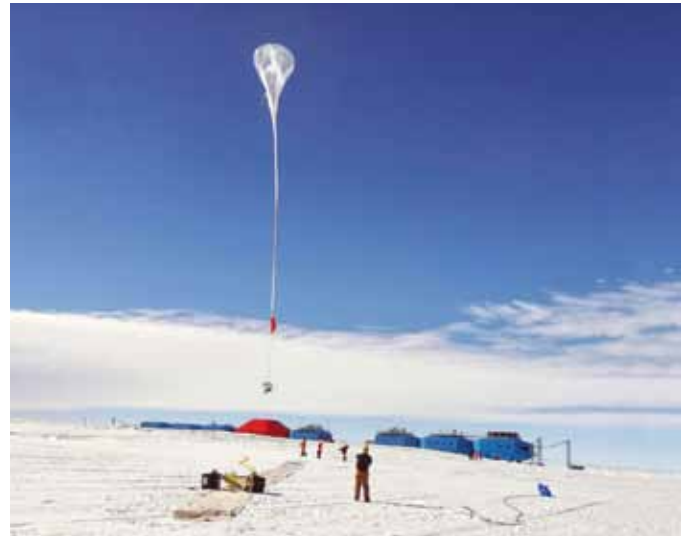
NASA launched the Balloon Array for Radiation-belt Relativistic Electron Losses (BARREL) over Halley Research Station in February 2014 to float above Antarctica and observe magnetic fields to augment measurements from the Van Allen Probes spacecraft. Image Credit: NASA
