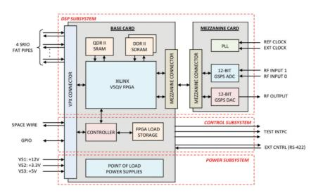
A 3U SpaceVPX programmable wideband transceiver/ processor adaptable to radar, scatterometry, and radiometry applications.
