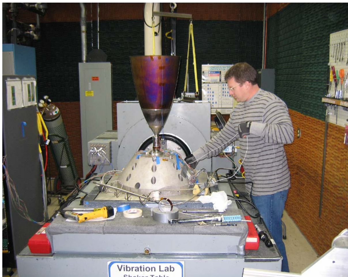
Setting up AMBR Engine for Vibration Test at Aerojet, Redmond
